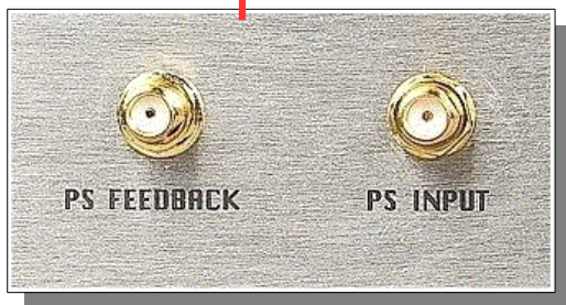
PureSignal connectors (usually looped together at factory)
