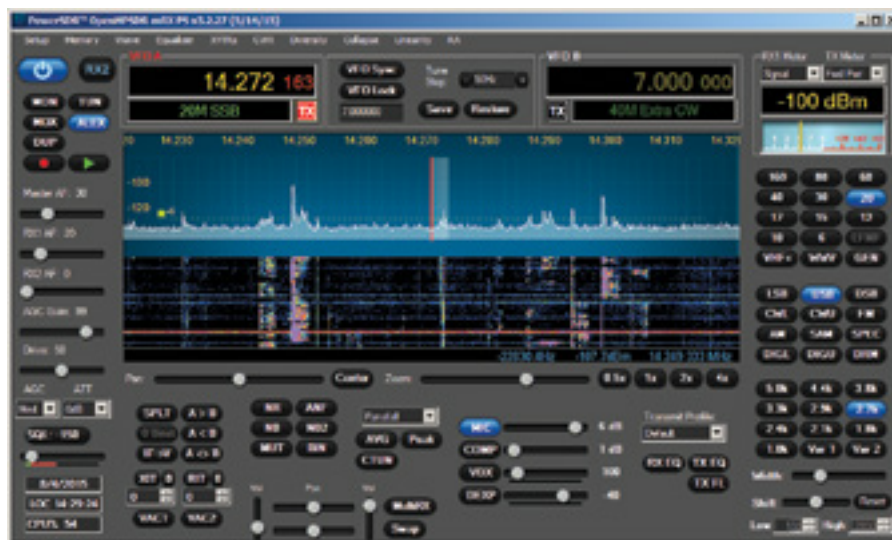
Figure 5 — PowerSDR offers spectral and waterfall displays, along with access to all transceiver functions.
