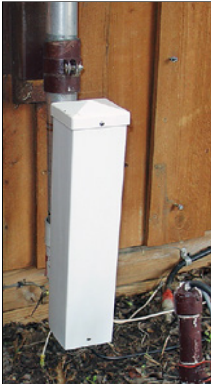
Figure 7 — MFJ-2910 connected to the base of the reviewer's 43-foot vertical.
