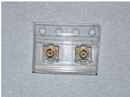
**4. Solder the Micro Coaxial Connectors J28, J29 on the top layer of the Hermes PCB (supplied with the Kit)**
