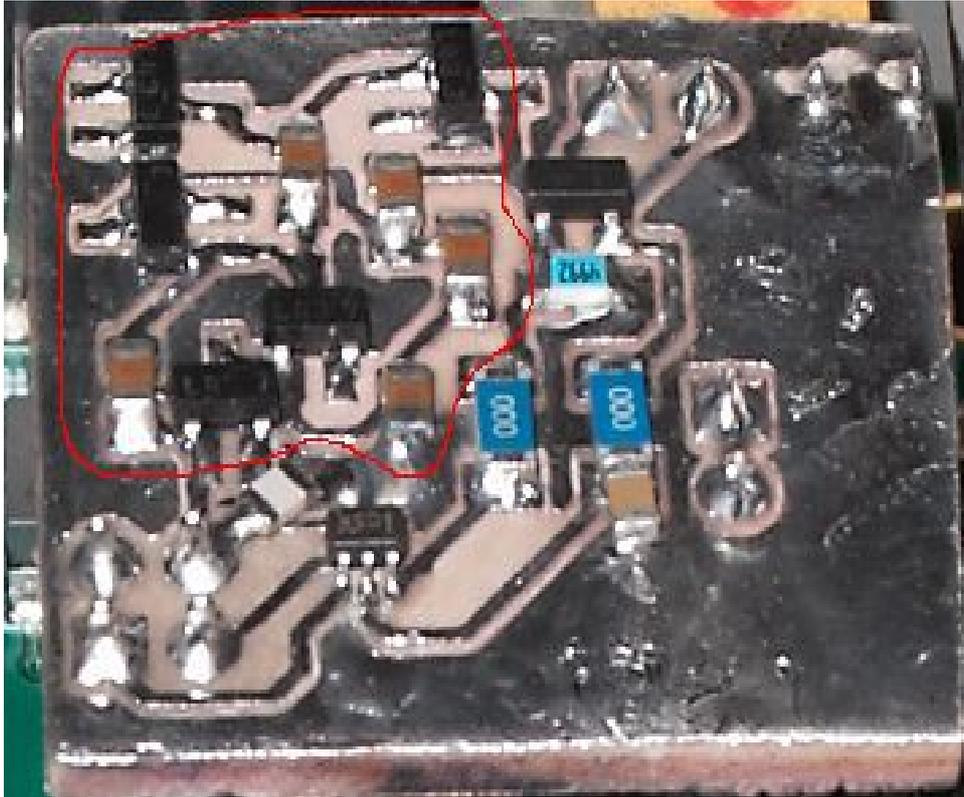
The output is loaded with 49K or so to control switcher time to INT10MHZ. (No load took many seconds to switch).
