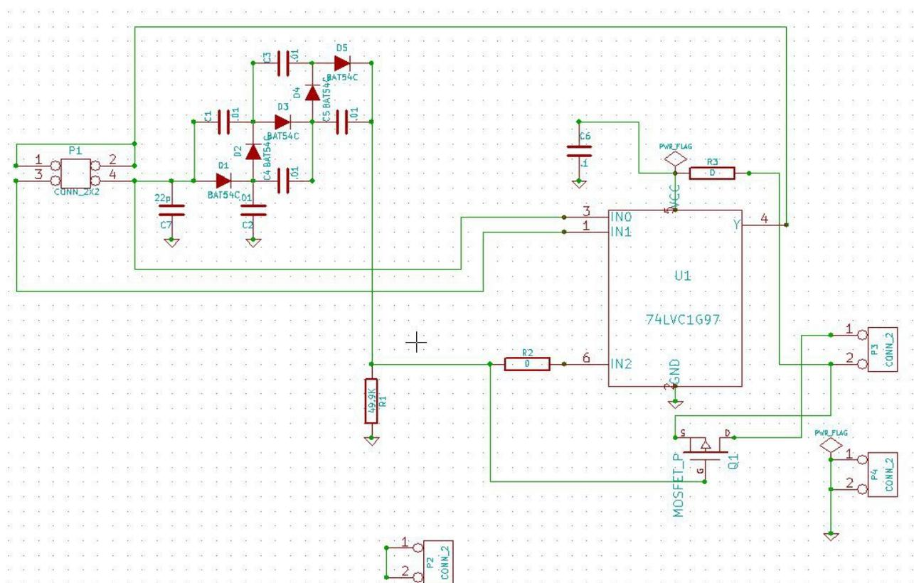
The detector would need to drive the select line and also enough voltage for use as a gate drive for a P channel power SW for the power feed to the INT10MHz oscillator.
