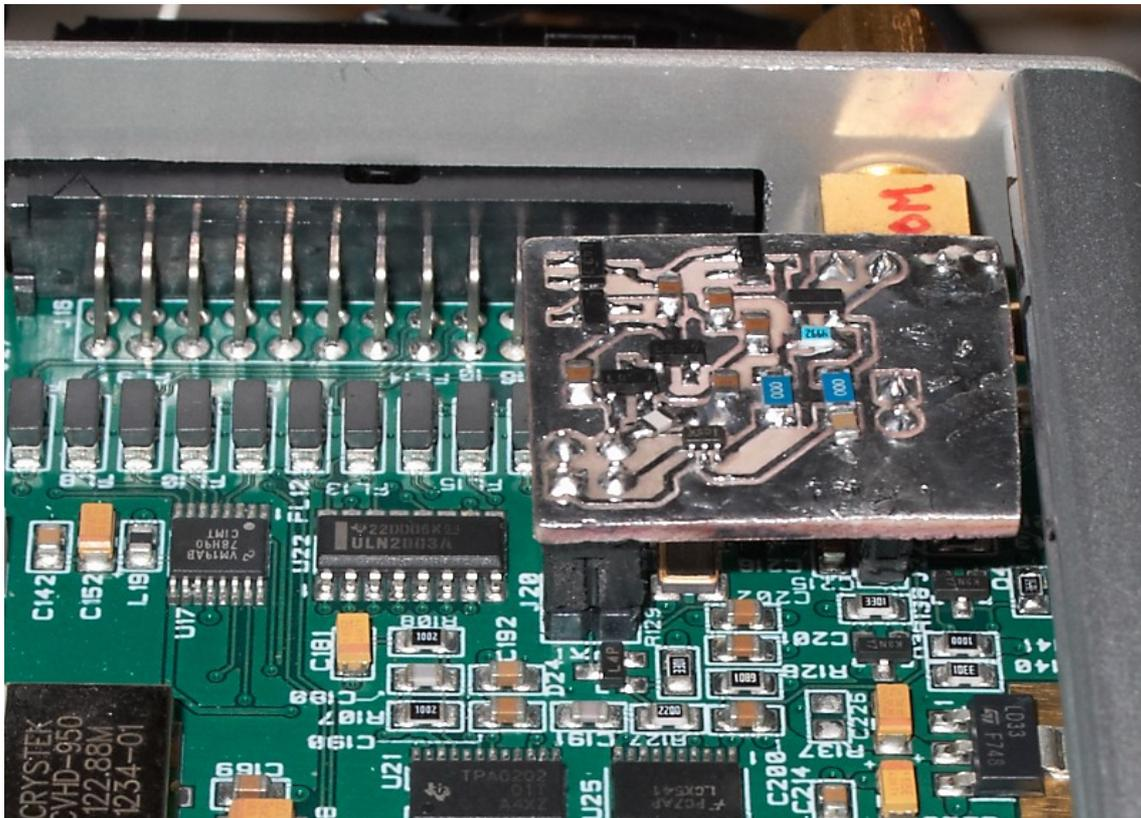
Recently, I built a small schmitt trigger buffer board for taking the slow edge speed 10MHz signal from the differential pair circuit in the Hermes. This buffer eliminated the "slips" when using the external 10MHz. Many users have sent me emails asking if I could come up with a autoswitched version which would use the internal 10MHz TXCO if the external signal is not present. Here is a list of possible improvements with a new Autoswitched design:
