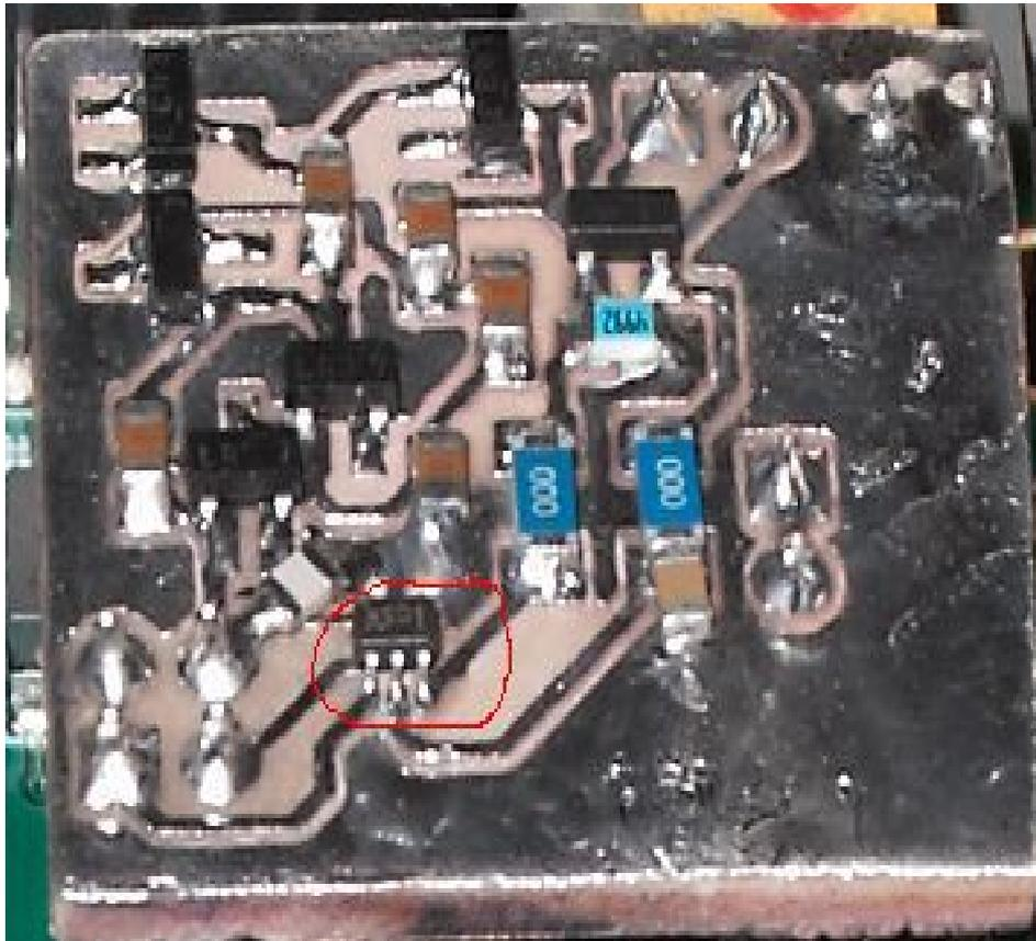
Also the signal is used to drive the gate of a P-ch Mosfet (source at 3.3V, and drain to power INT10MHZ oscillator).
