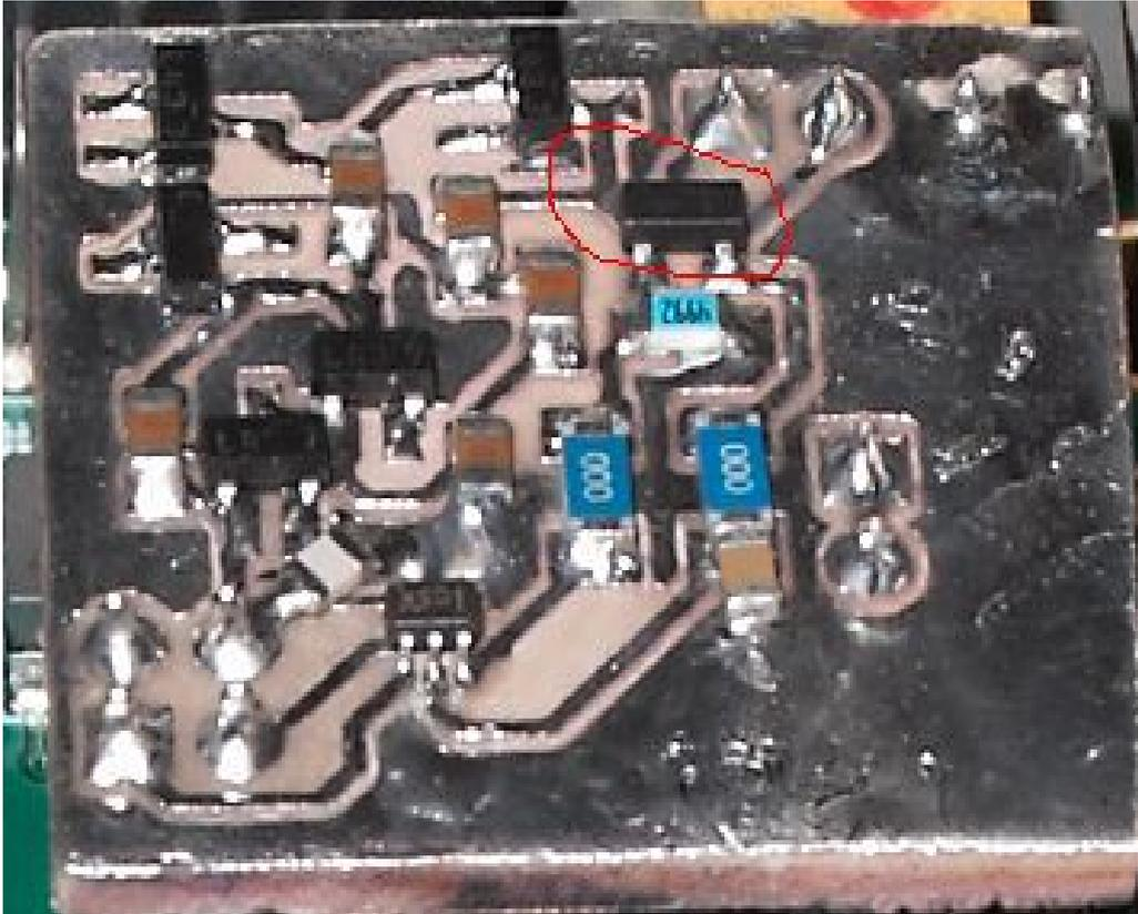
Circuit was simulated with LTSpice and a rough 1" X .7" single sided Layout was done on KICAD. A prototype was manually etched and built (wrong diode footprint so used leaded ones :)). The prototype seems to work perfect. Switches back and forth in a sec or so. The loaded control voltage is measured just above 3V or so providing good swing for the MUX and FET.
