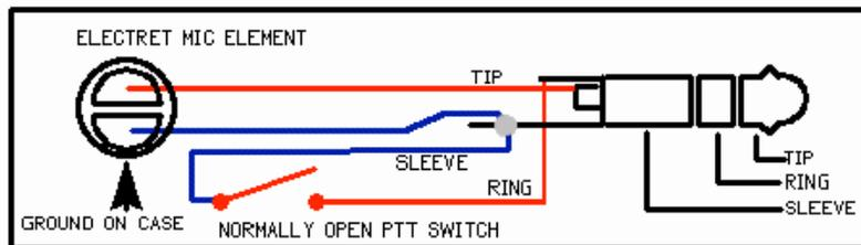
To select the tip for the mic audio, place the jumper on **JP4 pins 2 and 3 (default)**; to select the ring, use pins 1 and 2.
